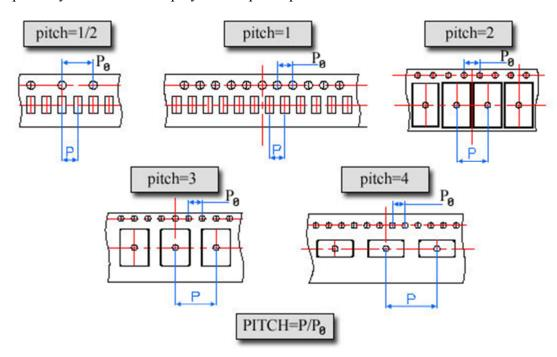
It can be seen that pitch equals the number of puncture holes between two parts (gaps between two holes are 4mm on all tapes). **PRESET** key: Press this key and enter the desired number. The
