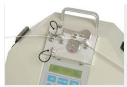
Model 2000PC shown with pocket check feature that transmits light through any pocket on plastic tape that's missing a component.
